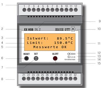
The different operating conditions are signalled via the status display and the fault signal light.
